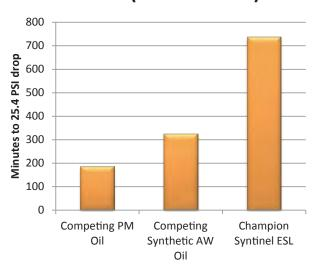
Outstanding oxidative stability ensures long fluid life and reduced service intervals, resulting in lower maintenance labor costs and higher productivity. High oxidation resistance also reduces the buildup of sludge and varnish on components.
